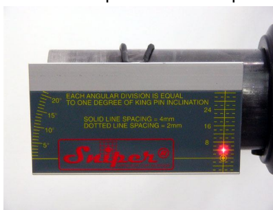
Rear Targets for measuring Chassis Twist, Squareness and Compound King Pin Inclination.
